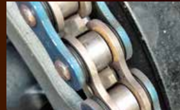
dry surface, lack of lubrication
