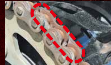
insufficient lubrication, roller wear
