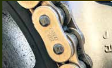
no rust, good condition
